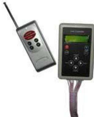
**Electronic Digital RF Flexible strip controller 5Volt DC
