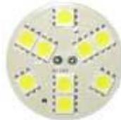
**G4 JC 9 SMT 5050 (3 Chip) Forward Firing Low Voltage 12V
