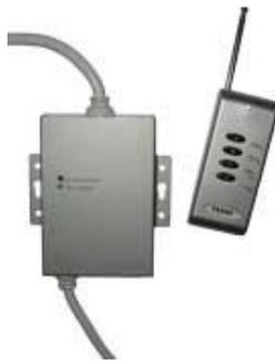
**Radio Controlled RGB LED Light Controller 12 Volt
