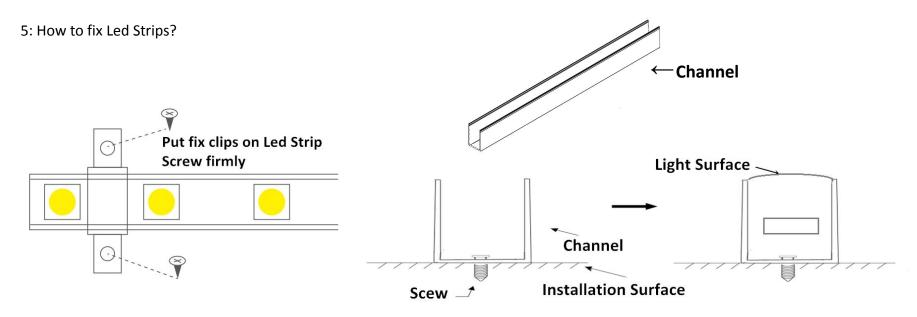
Three options for fixing Led Strip: ① Plastic Fix Clips; ② Plstic channel; ③ Aluminum channel.
