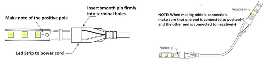
NOTE: Please apply glass glue at every connectors to make sure waterproof after checking Led Strip work properly.
