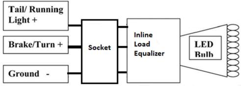
Please connect the inline load equalizer in between your female socket and the led bulb without cutting your existing wires.
