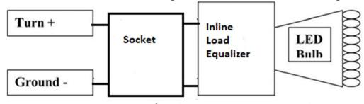
1154, 1157, 1158, 7443 and 3157 dual filament installation drawing:
