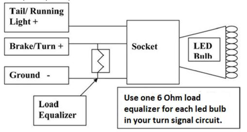
Please use the supplied insulation displacement crimps to connect the load equalizer in parallel with your led bulb without cutting your existing wires.
