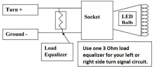
1154, 1157, 1158, 7443 and 3157 dual filament installation drawing:
