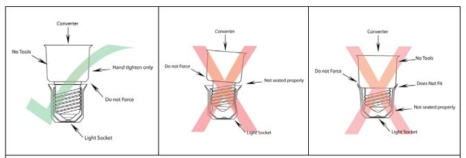
If the converter does not physically fit in to the light socket (contacts are not touching, or contacts are shorted and not properly seated.). This will cause the light bulb screwed into the converter not to work or cause damage. Please do not force the converter in to the light socket or it will cause damage to the converter, light bulb or light socket. Remove the converter and contact www.LEDLight.com for further support.
