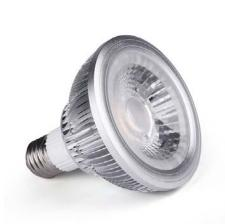
10 Watt MCOB LED PAR30. Uses only 10watt, comparable to a 60 watt light bulb. E27 Base. Uses MCOB technology, for the newest in LED Lighting technology. ETL Listed. White 6000K, Warm White 3000K, Red(625nm), Green(526nm), Blue(464nm),& Yellow(594nm).
